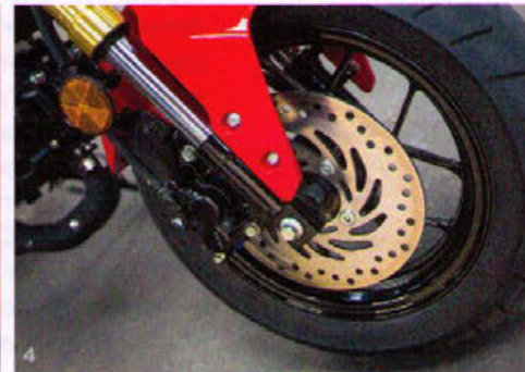
(1) Single Rear Shock, (2) Multi-Function Digital Instruments, (3) Stylized Bodywork, (4) Inverted Fork Suspension & 12-inch 10-spoke Wheels
